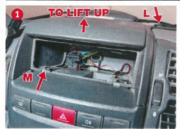
1. Remove the car radio, recover the two front screws M and the two rear screws L then remove the original panel.
