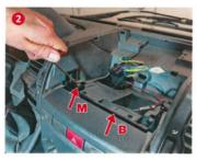
2. Place the "base bracket B" using the two screws original M.
