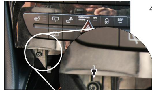
4. Remove the control unit / or CD-Changer underneath the OEM radio by removing the screws at left and right side
