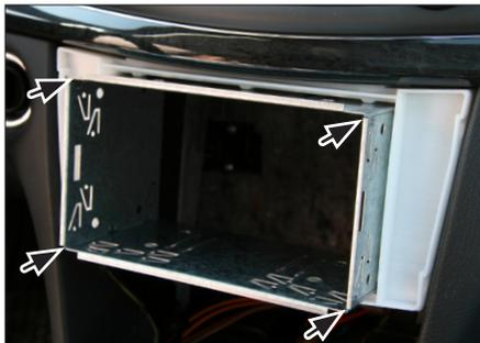
7. Push the metal frame into the mounting bracket
