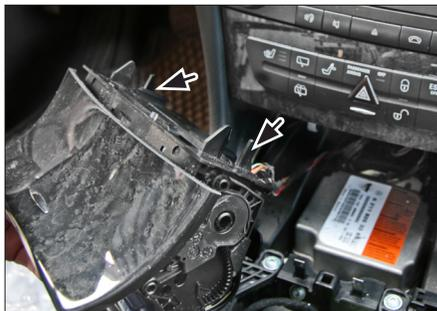
3. Open the ash tray and remove the complete ash tray unit
