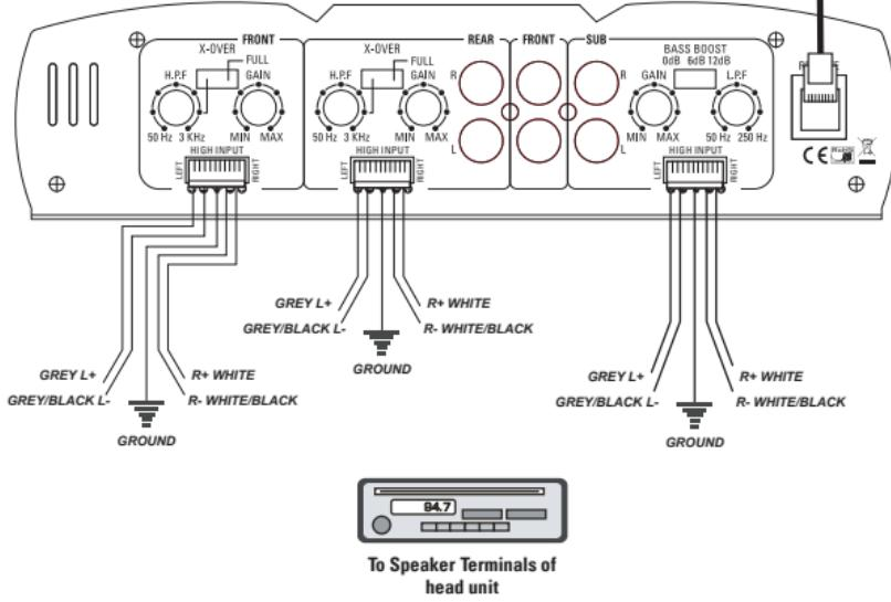
The high level input(s) should only be used if the RCA output are not present, connect the speaker outputs from the receiver to the high-level input connector of the amplifier. Be sure to observe polarity to avoid audio phase problems.
