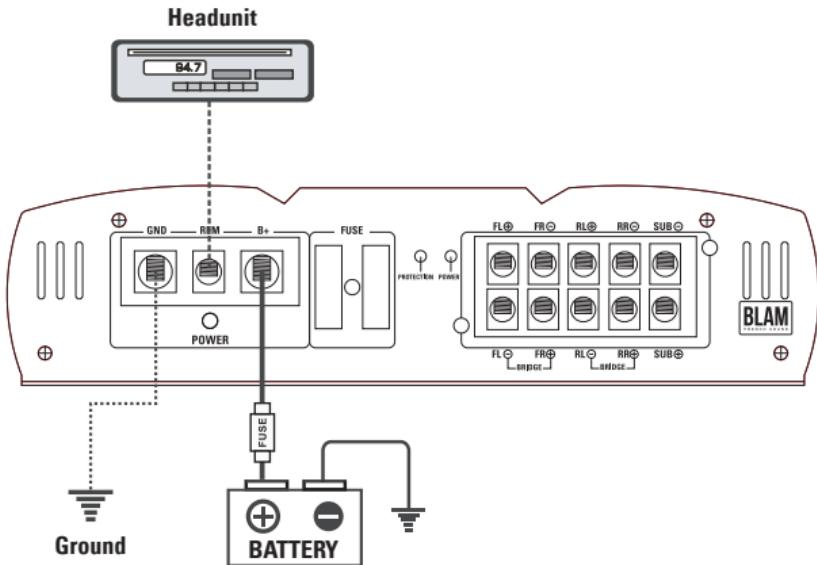
Connect an empty fuse holder within 18" [45 cm] of the car battery, and run 8 gauge [or heavier] cable from this fuse to the amplifier location. Then connect the fuse holder to the "BATT+".
