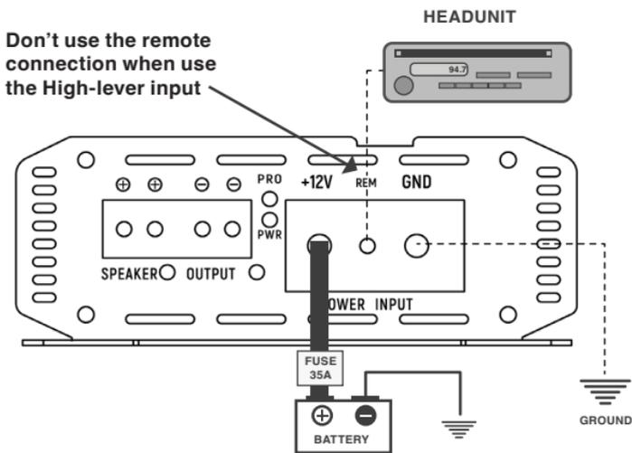
Connect an empty fuse holder within 18" (45 cm) of the car battery, and run 8 gauge (or larger) cable from this fuse to the amplifier location. Then connect the fuse holder to the "BATT+". Connect the ground terminal to the closest point on the chassis of the vehicle. Keep this ground wire to less than 39" (100 cm) in length. Ensure that the contact surface is free of paint or rust so that the connection between the terminal and the chassis is effective.
