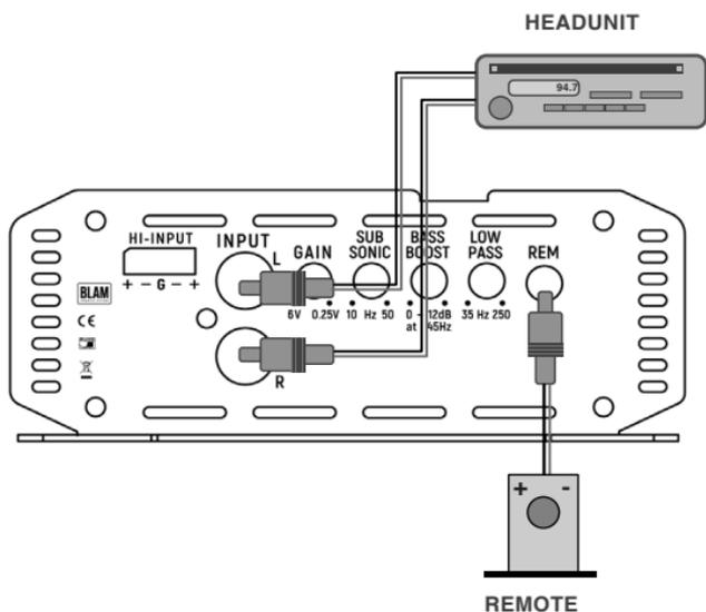
Low-level (RCA) Input wiring is preferred for best audio performance. Most trunk or hatchback installations will require a 15-20 feet RCA cable, while pickup trucks and under-seat Installations will require a 6-12 feet RCA cable. Always use a high quality cable. Connect to remote turn on terminal head unit.
